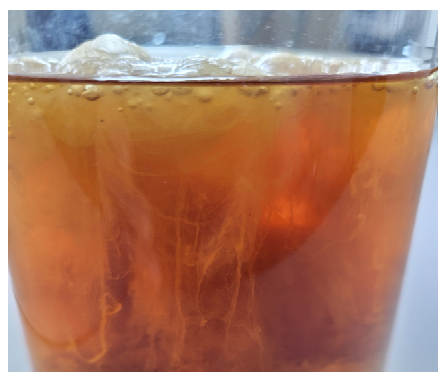
Figure 1: coagulation – formation of lumps by mixing two incompatible foam concentrates
